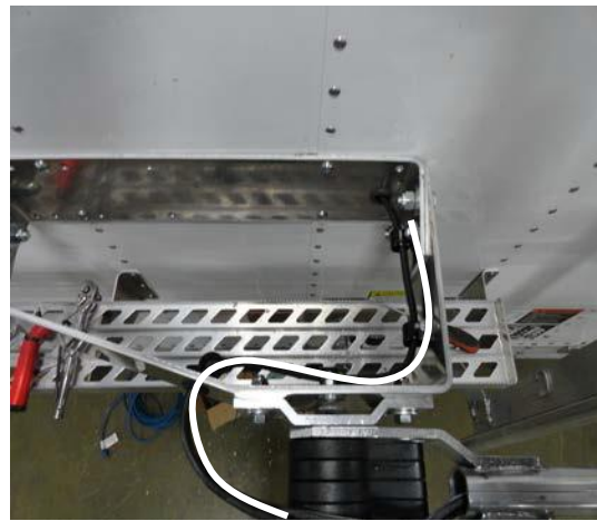
Suggested Wire Routing using the Universal Bracket (White Reference Line)
